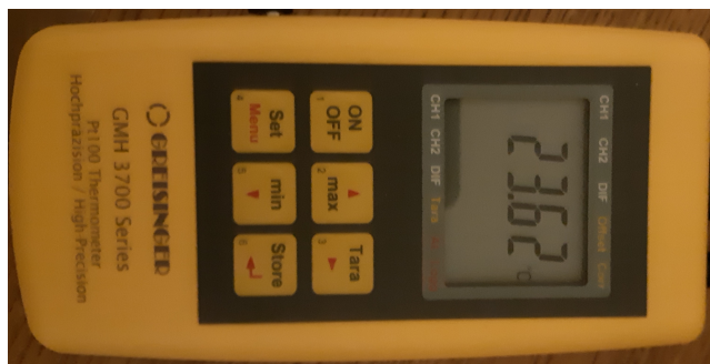
Figure 18: Reference Sensor Greisinger GMH 3750
